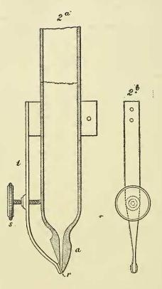
dered on. It is made sufficiently large to admit of variation in the diameter of the burette tubes, a strip of paper being used as a filling. The delicacy of the hinge, and to some extent the cost of the apparatus (\$2.50) have prompted me to substitute a simpler construction.
